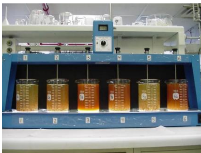
Image 6. Jar Test equipment (Sigmada)
